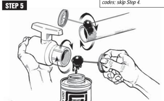
VALVE INSTALLATION CAUTION: Take extra care that no primer or solvent cement is allowed to contact the ball or other internal valve components.
