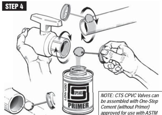
NOTE: CTS CPVC Valves can be assembled with One-Step Cement (without Primer) approved for use with ASTM D2846 products. Check local codes; skip Step 4.
