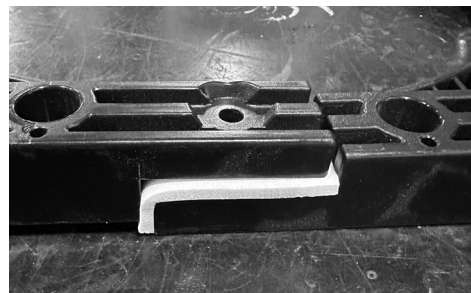
Image 7 Foam Strip Installation
