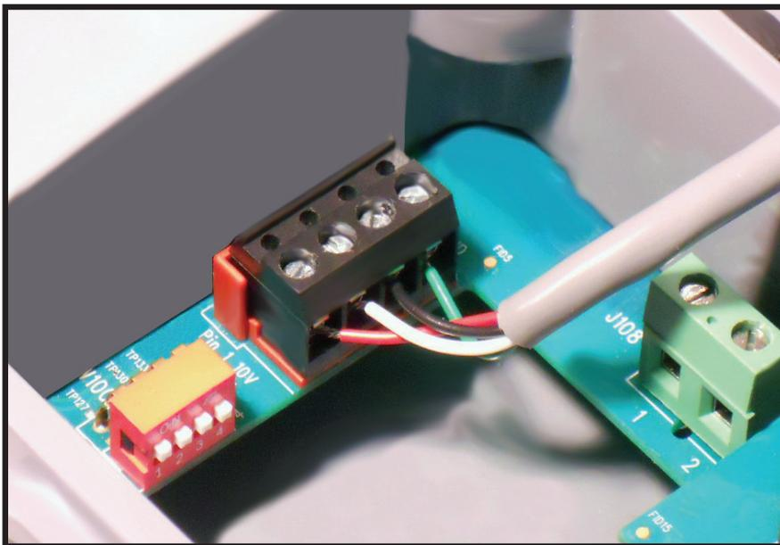
**Figure 14: UI connector installed**
