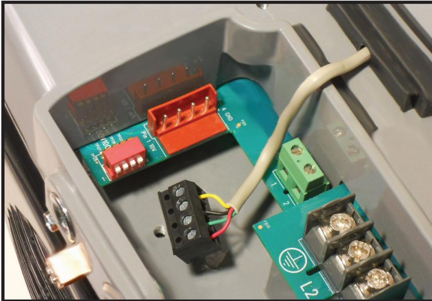
**Figure 13: Communication Connector Removed**
