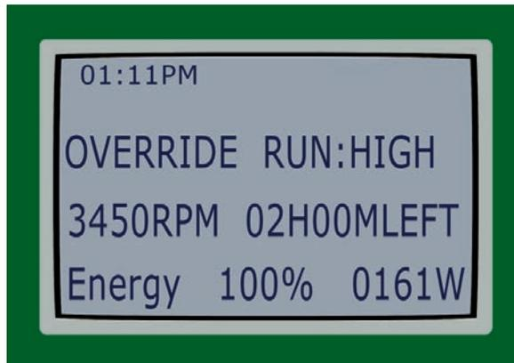
The Override High button can program the motor to temporarily run at speeds between 600 and 3450 RPM. Override High is recommended for high flow uses such as a pool heater startup, backwash, filtering, and cleaner water requirements that exist outside of the daily operating schedule. Once the Override High duration is completed, the motor will automatically return to the programmed schedule.
