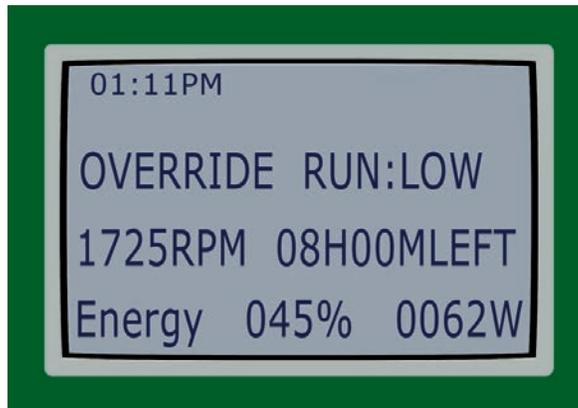
The Override Low button can program the motor to temporarily run at speeds between 600 and 3450 RPM. Override Low is recommended for low circulation requirements that exist outside of the daily operating schedule. Once the Override Low duration is completed, the motor will automatically return to the programmed schedule.
