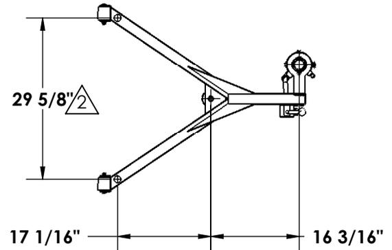
△<sub>2</sub> Note: Clear deck space shall be provided parallel to the water 36" wide x 48" minimum from a line located 2" behind the rear edge of the seat. (15.8.5.3 ADA Guidelines)
