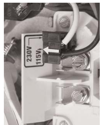
Figure 5B -Voltage Change Plug Set for 115 Volts
