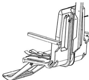
18. Attach foot rest to seat with bolts and thumbnuts.
