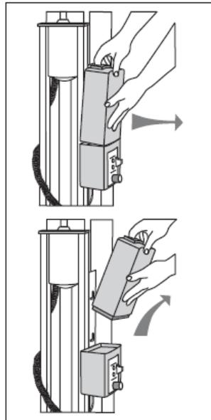
**To remove** - pull the battery pack away from the mounting plate so that the latch on the battery pack clears the side tabs on the mounting plate - then lift the battery pack up and away from the Control Box.
