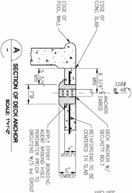
NOTE: VERIFY THE SLAB THICKNESS AFTER CURING. DO NOT INSTALL IF SLAB IS LESS THAN 4" THICK.
