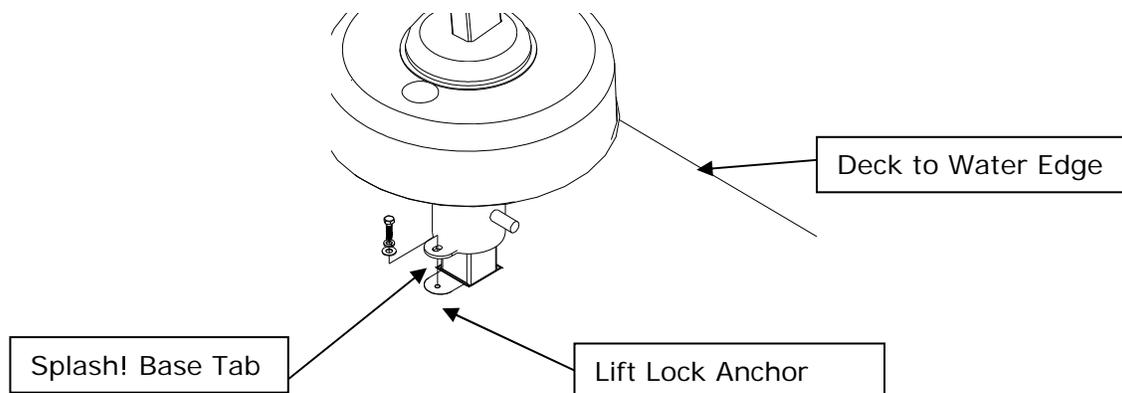
5. Position the mast assembly onto the housing cover by lowering the mast base onto the studs protruding from the housing. Attach the washers and lock nuts onto the studs and fully tighten using a 3/4" or 19mm socket wrench. Slide attachment cover to cover the bolts.
