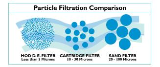
The System 3 Mod D.E. filter also has a clear advantage over traditional-style D.E. filters:
