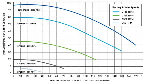
NOTE: The chart above demonstrates performance rates at factory preset speeds of 750 RPM, 1500 RPM, 2350 RPM and 3110 RPM.
