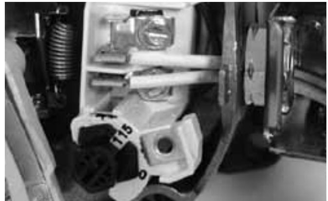
**Figure 7: Voltage set to 115 volts, Dial Type**
