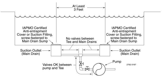
Figure 2 – Recommended pump suction layout.
