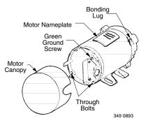
Figure 3: Typical ground screw and bonding lug locations.
