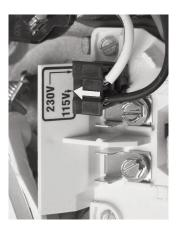
Figure 5A -Voltage Change Plug Set for 230 Volts
