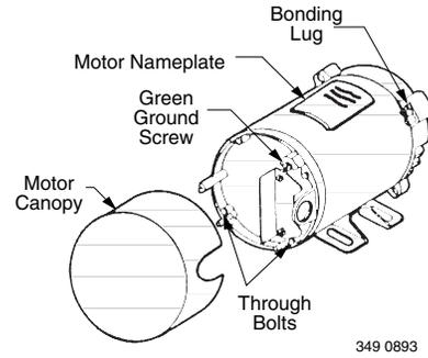
Figure 3: Typical ground screw and bonding lug locations.
