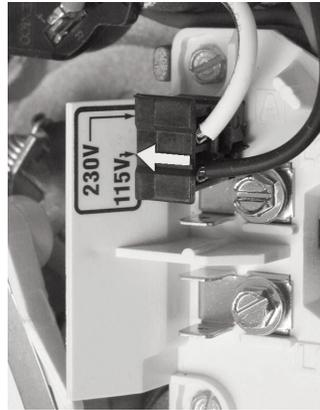
Figure 5B Voltage Change Plug Set for 115 Volts
