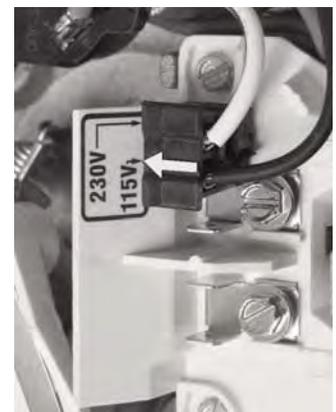
Figure 4B Voltage Change Plug Set for 115 Volts
