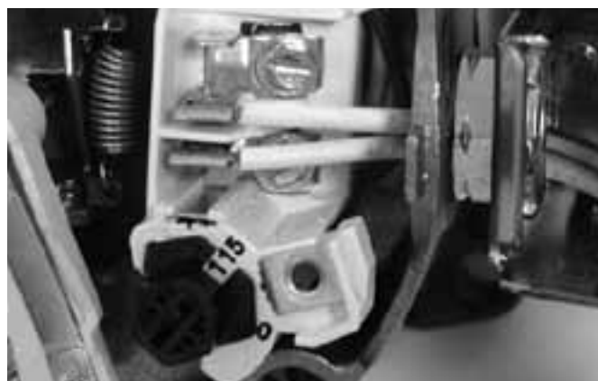
Figure 11: Voltage set to 115 volts, Dial Type
