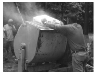
Because FDD is in a dry, powdered state, excessive dry mixing would lose valuable additives to the air, while mixing wet would cause FDD to float. Total water content (per unit) should not exceed 8 gallons. If additional water is necessary, the sand is too fine. Caution: the use of sand other than marble sand will cause the finished FDD to be hot.
