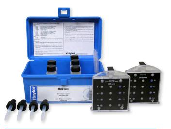
Unless the sample appears colored or turbid, a Midget comparator may be used to determine the concentration of metal in the water. K-1264 is shown.
