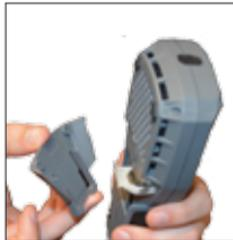
1. To install battery, remove rear battery compartment cover. Insert one CR2032 battery into compartment. Replace battery compartment cover.
