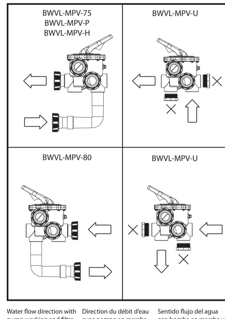
Water flow direction with pump working and filtration position.
