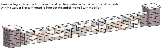
This page shows typical construction details for Belvedere walls. These drawings are representative of major components required in wall construction. Specific details including geotextile reinforcement layers, drainage details, soil requirements, etc. shall be per engineered design for the wall.
