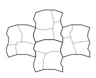
Note: Outside dimensions of each layer are identical to all other layers, allowing any layer to be substituted anywhere in the pattern.
