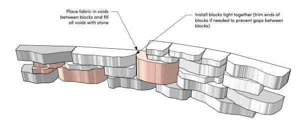
This page shows typical construction details for Outcropping walls. These drawings are representative of major components required in wall construction. Specific details including geotextile reinforcement layers, drainage details, soil requirements, etc. shall be per engineered design for the wall. For more cross-section and design options, visit our website.
