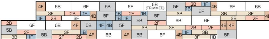
Note: 2 in (51 mm) must be trimmed from (1) 18 in X 6 in (457 x 152 mm) block to make this pattern
