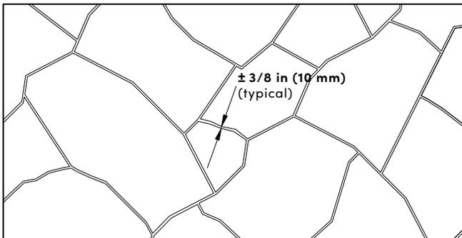
Individual pieces of Grand Flagstone can crack either during delivery to the job or during on-site handling prior to placement. Typically less than 5% of the pieces will crack. There are two methods to deal with cracked pieces.
