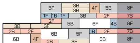
Note: For left and right ends, vertical end jogs in and out approximately 1 in (25 mm) between blocks.
