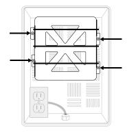
Remove the T100/A.1x bracket by removing the 4 screws that are securing the bracket to the enclosure plate.
