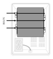
5. Loosen the horizontal bolts until they move up and down freely and insert the T100. Secure the T100 to the enclosure plate using the included velcro. Tighten the bolts to securely fasten the T100 in place.
