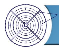
Internal ribs and walls are designed to optimize the impact-reducing capabilities of the disc, while keeping weight to the requisite level.
