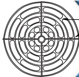
Internal ribs and walls are designed to optimize the impact-reducing capabilities of the disc, while keeping weight to the requisite level.
