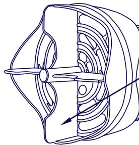
Four fins on both sides of the disc extend fully to engage with adjacent fins, thereby creating a solid wave-retention barrier. No water gets through.
