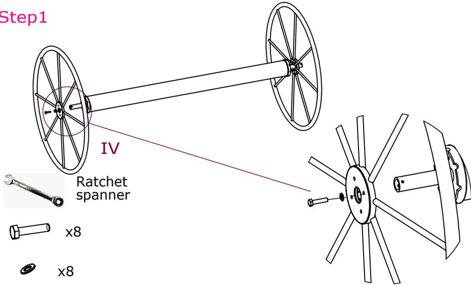
Use M10x45 Hex Bolts and Washers to fix the 2 Discs to both ends of the AXLE
