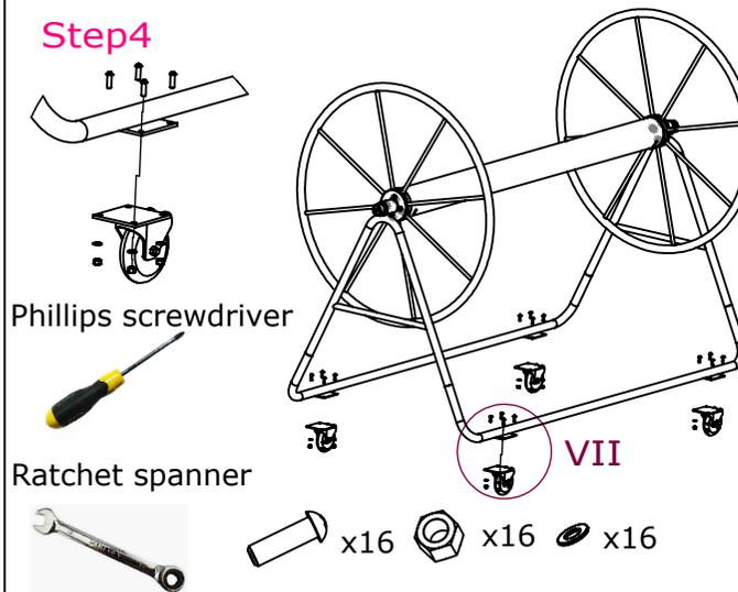
Use M8X20 Round Head Bolts, Washers and Lock Nuts to fix the Caster Wheel to the plate of "U" Frame, then place the Cover over the StoReel.
