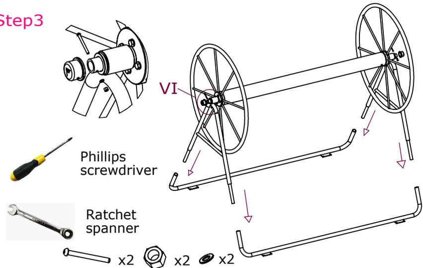
Put the "U" Frame on the ground as above, connect the "A" Frame and the "U"Frame, then use M6X80 Round Head Bolts, Washers and Lock Nuts to fix the Axle Cap to both ends of the Axle.
