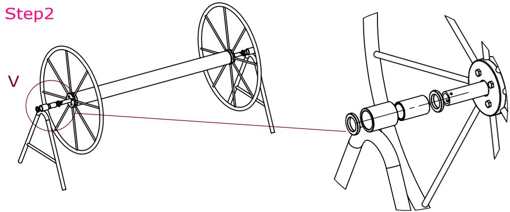
Slip the Nylon Washer, Nylon Bush, the top tube of "A" Frame and Nylon Washer on both ends of the Axle.
