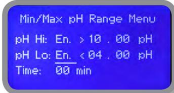
Move wheel on "pH Hi: Dis." and change status from "Dis." (option disabled) to "En." (option enabled) by clicking on wheel and rotating it. Press wheel again and move on next field. Press wheel and enter a value for HIGH alarm.
