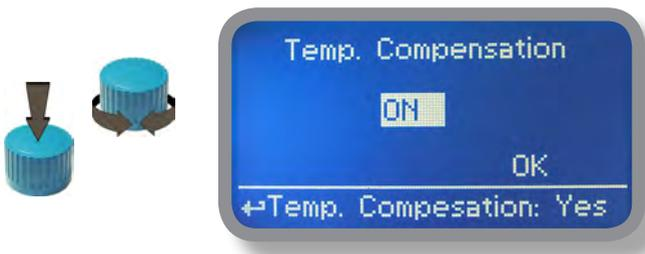
To end procedure move cursor on "OK" and press wheel to proceed to "Save" request screen. Move wheel on "YES" to save or "NO" to discard changes.
