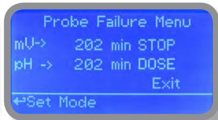
E.g. To set ORP pump to stop after time ends and probe doesn't change reading values press wheel, choose maximum time, press wheel move on next field and choose "STOP". Time can be set between 100 and 254 minutes. When satisfied with settings move on exit and press wheel.
