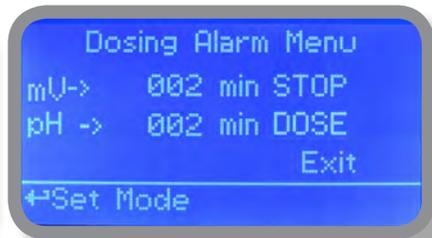
E.g. To set ORP pump to stop after time ends and setpoint isn't still reached press wheel, choose maximum time, press wheel move on next field and choose "STOP". Time can be set between 0 and 100 minutes. When satisfied with settings move on exit and press wheel.
