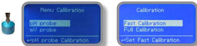
Fast Calibration procedure involves one point calibration (choose value closest to real field application).
