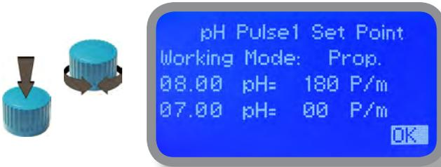
**PROPORTIONAL mode between 7pH(0 P/m) and 8pH (180 P/m).** p/m is : pulses per minute
