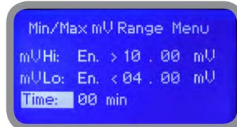
Move wheel on "mV Hi: Dis." and change status from "Dis." (option disabled) to "En." (option enabled) by clicking on wheel and rotating it. Press wheel again and move on next field. Press wheel and enter a value for HIGH alarm.
