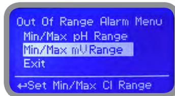
Move wheel on "Min/Max mV Range" to set "out of range" condition for ORP probe then click on wheel to enter into "Min/Max Range menu".
