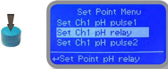
Proportional mode set the instrument to operate using a calculated percentage between two set values that enable or disable the pH pump. To use this mode move cursor on "Working Mode". Press the wheel and select it.
