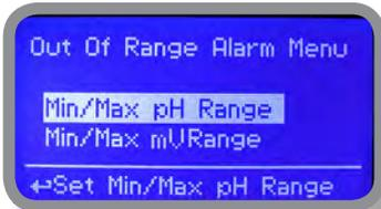
Move wheel on "Min/Max pH Range" to set "out of range" condition for pH probe then click on wheel to enter into "Min/Max Range menu".
