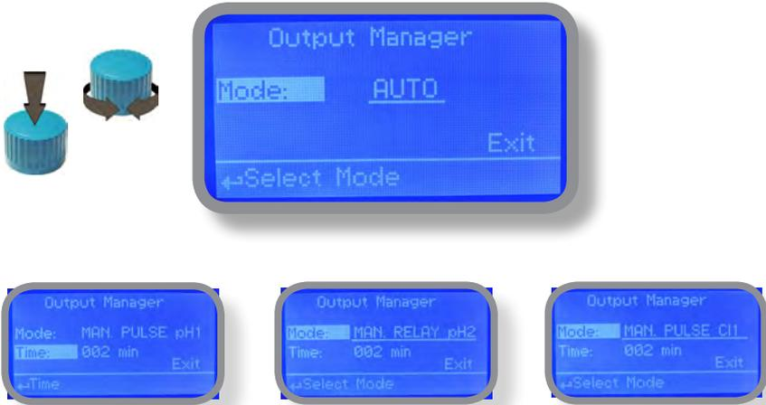
Press wheel to move cursor on "TIME" field. Once here, choose a working time between 0 (disabled) or 199 minutes. Move on "EXIT", then press wheel.
