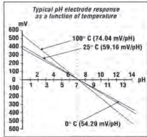
Instrument has either fixed or adjustable automatic temperature compensation referenced to a standard temperature of 25°C.
