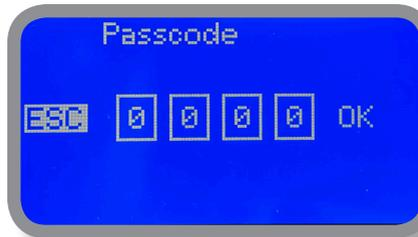
To set a new passcode choose "PARAMETERS" from "Main Menu", move on "New Pcode", click on wheel and enter a four numbers code. Click on "EXIT" and choose "YES" to save request. The new passcode is now ready.
