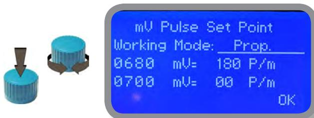
**PROPORTIONAL MODE between 700(0 P/m) and 680 (180 P/m). [P/m: pulses per minute]**
