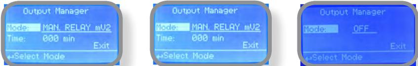
Exit from main menu. Main display will show a countdown for selected output. To stop this countdown go back to "Output Manager" menu and choose "AUTO" as working mode or wait until countdown ends. **This function can be used for priming purposes.**
