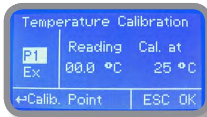
**Note:** This procedure assumes that instrument is correctly configured and properly connected to a working PT100. Calibrate using plant's temperature otherwise unattended results may occur.
