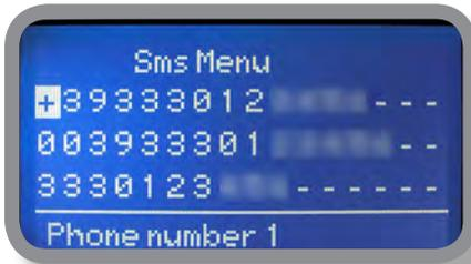
Up to three numbers for sending SMS can be stored into LDPHRH memory. SMS recipient will receive an SMS containing instrument ID, NAME and status. Number formats can be stored using international prefix "+", international prefix "00" or local.
