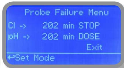
E.g. To set CI pump to stop after time ends and probe doesn't change reading values press wheel, choose maximum time, press wheel move on next field and choose "STOP". Time can be set between 100 and 254 minutes. When satisfied with settings move on exit and press wheel
