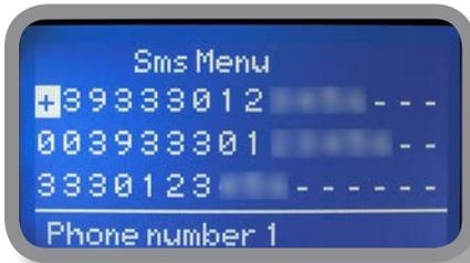
Up to three numbers for sending SMS can be stored into LDPHCL memory. SMS recipient will receive an SMS containing instrument ID, NAME and status. Number formats can be stored using international prefix "+", international prefix "00" or local.
