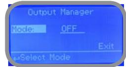
Main display will show a countdown for selected output. To stop this countdown go back to "Output Manager" menu and choose "AUTO" as working mode or wait until countdown ends. This function can be used for priming purposes.
