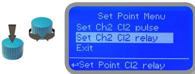
Proportional mode set the instrument to operate using a calculated percentage between two set values that enable or disable the Chlorine pump. To use this mode move cursor on "Working Mode". Press the wheel and select it.
