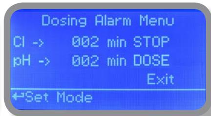
E.g. To set CI pump to stop after time ends and setpoint isn't still reached press wheel, choose maximum time, press wheel move on next field and choose "STOP". Time can be set between 0 and 100 minutes. When satisfied with settings move on exit and press wheel.
