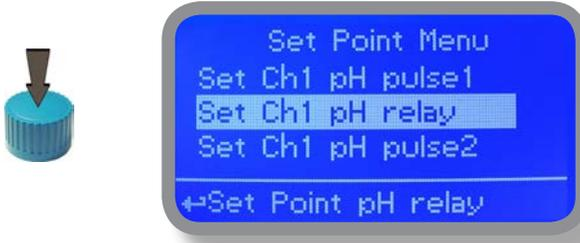
Proportional mode set the instrument to operate using a calculated percentage between two set values that enable or disable the pH pump. To use this mode move cursor on "Working Mode". Press the wheel and select it.
