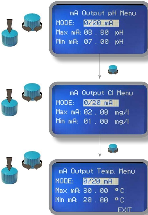
Rotate wheel to move within all 3 channels. Click wheel to select parameter and rotate wheel to change it. Click wheel again and rotate wheel to move cursor on next parameter. To end procedure move cursor on "EXIT" and press wheel to proceed to "Save" request screen. Move wheel on "YES" to save or "NO" to discard changes.
