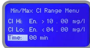
Move wheel on "CI Hi: Dis." and change status from "Dis." (option disabled) to "En." (option enabled) by clicking on wheel and rotating it. Press wheel again and move on next field. Press wheel and enter a value for HIGH alarm.
