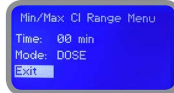
As last option enter "Time" (max 99 minutes) after which if lower or higher read value condition stays then the alarm occurs (to set into mode field)
