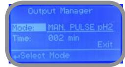
Press wheel to move cursor on "TIME" field. Once here, choose a working time between 0 (disabled) or 199 minutes. Move on "EXIT", then press wheel.
