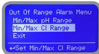
Move wheel on "Min/Max CI Range" to set "out of range" condition for Chlorine probe then click on wheel to enter into "Min/Max Range menu".
