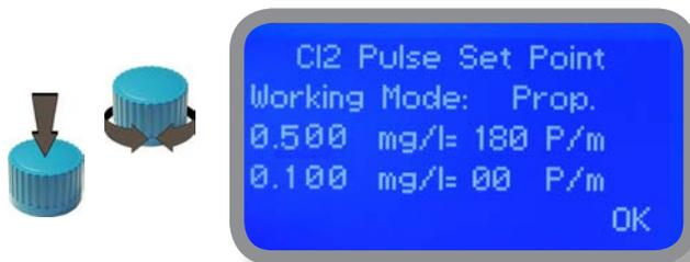
**PROPORTIONAL mode between 1.00Cl (0 p/m) and 0.50Cl(180 p/m). p/m is : pulses per minute**
