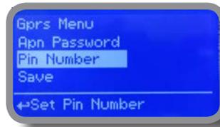
Instrument can be set for ERMES services enabled (Configuration option set to “ERMES YES”) or messages only (Configuration option set to “ERMES NO”) based on your SIM data access parameters. For manual configuration option enter APN (access point name) and SIM phone number. Move wheel on “OK” to save and move on “ESC” to go back to main menu.
