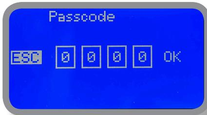
To set a new passcode choose "PARAMETERS" from "Main Menu", move on "New Pcode", click on wheel and enter a four numbers code. Click on "EXIT" and choose "YES" to save request. The new passcode is now ready.
