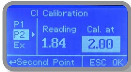
Fast Calibration procedure involves one point calibration (choose value closest to real field application)
