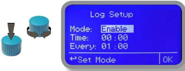
Log activity recording can be started by moving wheel on "Mode: Disable" and changing it to "Mode: Enable". Log activity starting time can be set to begin at specified time by entering "Time". Activities data are collected every specified hour or minute. Edit this parameter by moving wheel on "Every: 00:00" and changing it to desired time.
