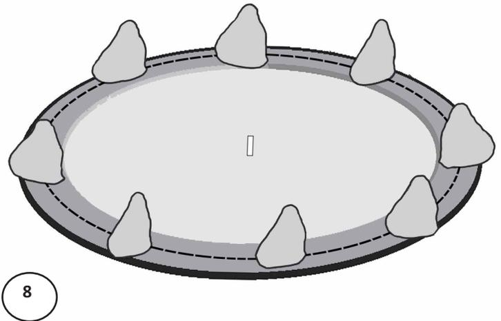
**Note:** Bottom rails will be placed in the center of the perimeter of the pool see the dashed line. *(Image 8)*
