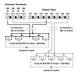
Refer to sample diagram. Connect one side of fixtures (common) up to 300 watts per circuit, using 12 gauge or larger direct burial cable. Strip 3/4" of cable insulation and twist wire strands tightly before insertion into transformer's output terminals. Each terminal will accept two #8, four #10, or 6 #12 wires. Tighten connector screws firmly. Retighten after one week of
