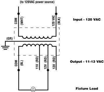
transformer. Timers and photocells must be installed in a remote location to the transformer, in line with the input supply wiring.
