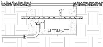
**NOTE:** Do not route low voltage cables through the same conduit as the line voltage supply cables.
