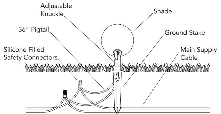
**The operating voltage range for this LED luminaire is 6 - 15 volt AC.** The Vista electronic driver ensures the LED operates at the intended lumen output while receiving voltage as low as 6 volts, and as high as 15 VAC, resulting in a balanced lumen output from the first fixture to the last. Eliminating the dimness issues often attributed to voltage drop.
