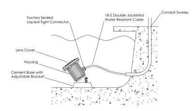
**The operating voltage range for this LED luminaire** is 6 - 15 volt AC. The Vista electronic driver ensures the LED operates at the intended lumen output while receiving voltage as low as 6 volts, and as high as 15 VAC, resulting in a balanced lumen output from the first fixture to the last. Eliminating the dimness issues often attributed to voltage drop.
