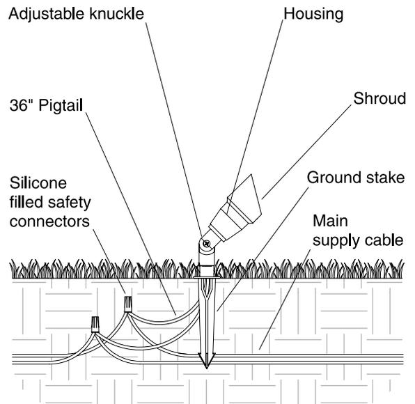
**The operating voltage range for this LED luminaire is 6 - 15 volt AC.** The Vista electronic driver ensures the LED operates at the intended lumen output while receiving voltage as low as 6 volts, and as high as 15 VAC, resulting in a balanced lumen output from the first fixture to the last. Eliminating the dimness issues often attributed to voltage drop.
