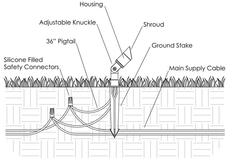
**The operating voltage range for this LED luminaire is 6 - 15 volt AC.** The Vista electronic driver ensures the LED operates at the intended lumen output while receiving voltage as low as 6 volts, and as high as 15 VAC, resulting in a balanced lumen output from the first fixture to the last. Eliminating the dimness issues often attributed to voltage drop.
