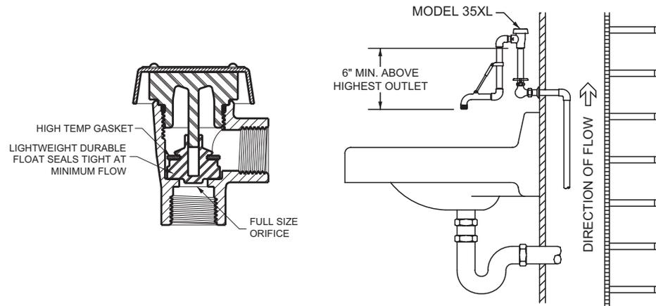
**CAUTION:** This device should never be used in installations that are under continuous pressure. Therefore, never place a shut-off or check valve downstream of AVB's. This device shall not be installed in a concealed or inaccessible location, nor where the venting water from the device during normal functioning may be deemed objectionable.
