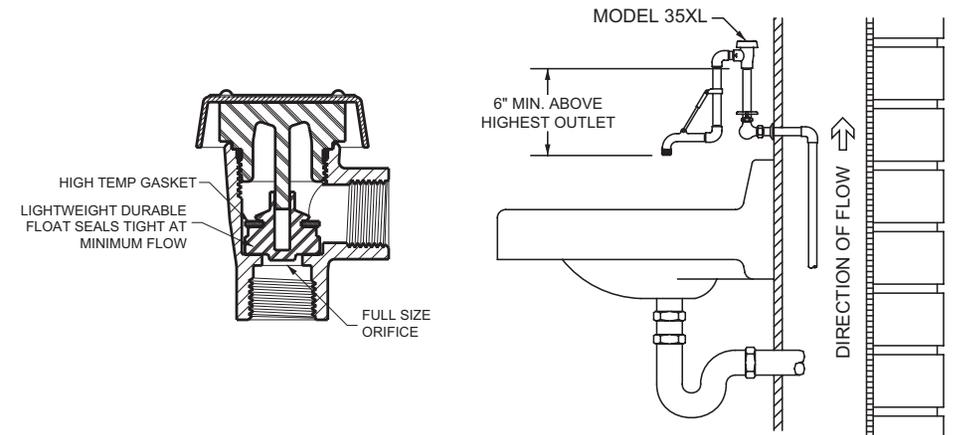
**CAUTION:** This device should never be used in installations that are under continuous pressure. Therefore, never place a shut-off or check valve downstream of AVB's. This device shall not be installed in a concealed or inaccessible location, nor where the venting water from the device during normal functioning may be deemed objectionable.
