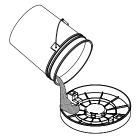
Insert supplied plaster shields. Pour the desired material into the fillable side of the lid.
