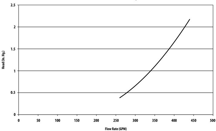
Head Loss Curve - Diamond Strip Drains
