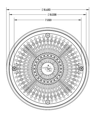
**Description** Part No. 819-0051 #8 Stainless Steel Screw - 32 x 5/8 642-2400 V 8" Tru Flo Drain Cover 642-214X 8" Tru Flo Drain Frame
